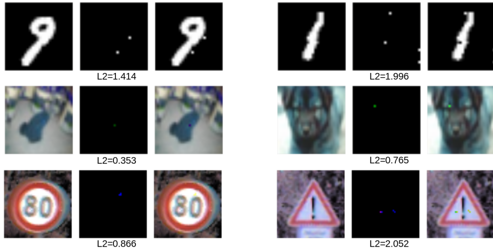
Figure 5.13: Examples of adversarial MNIST, CIFAR-10 and GTSRB images with slight perturbations based on the L^2 norm. Top: “9” misclassified into “8”; “1” misclassified into “3”. Middle: “frog” misclassified into “dog”; “dog” misclassified into “cat”. Bottom: “speed limit 80 mph” misclassified into “speed limit 60 mph”; “danger” misclassified into “pedestrian crossing”.
