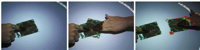
Figure 4. The duplicate coordination policy: when more than one user simultaneously grabs a document, a copy is automatically produced.
