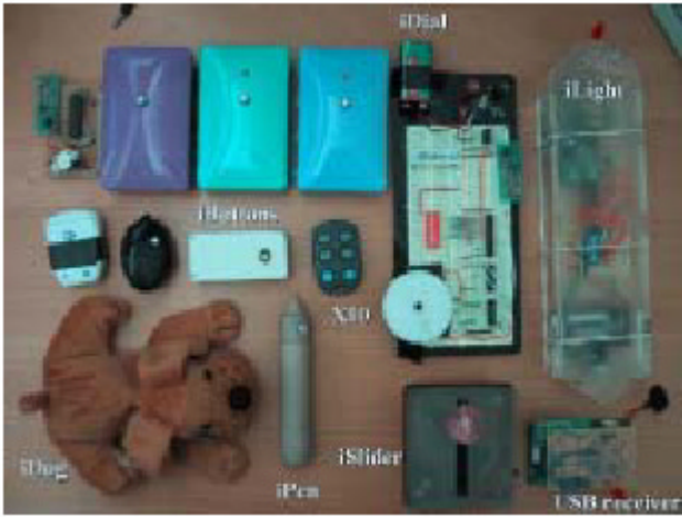
Figure 1. Various iStuff. The iDog sends a button press event when turned over. The iPen is an augmented SMARTBoard pen, where the embedded button operates as a “right click” to the Windows OS. The X10 buttons are standard X10 hardware. All other devices work through a simple RF receiver that plugs into the USB port of the Proxy PC.
