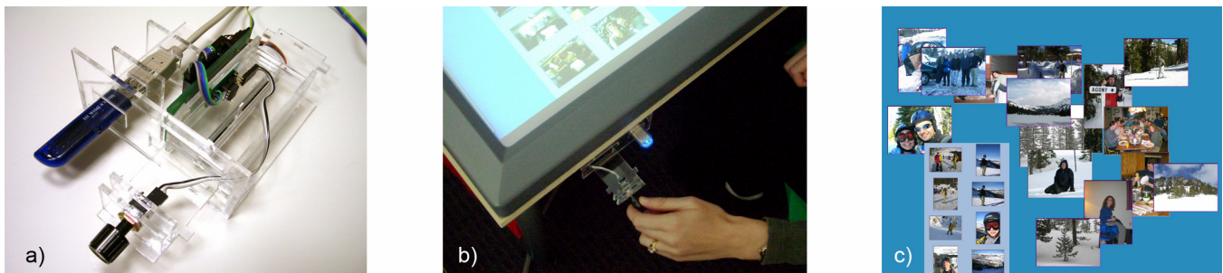
Figure 1. a) An acrylic drawer mechanism, connected to the PC via d.tools, affords pulling and pushing, as well as scrolling. The drawer has a slot for plugging in a USB flash drive. b) Four drawers are attached to the DiamondTouch table, one on each side. c) Pulling out the physical drawer handle opens a virtual drawer on-screen, which can be used to store data objects, such as the digital photos shown in the lower left corner here.
