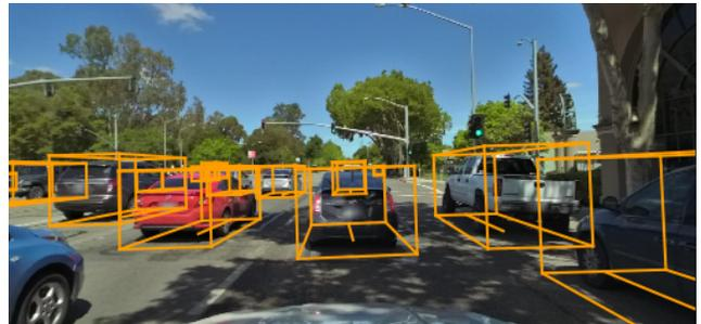
Figure 1: AV camera image with vehicle bounding-boxes [40]
