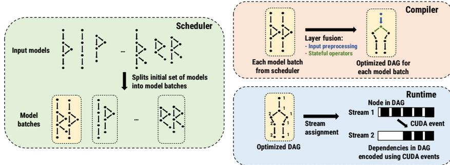
**Figure 2:** HiveMind’s proposed architecture. Input models are first grouped into model batches using HiveMind’s *scheduler*; each model batch is then optimized using HiveMind’s *compiler*; the optimized DAG is then executed on GPUs using HiveMind’s *runtime*, which makes use of the CUDA Stream and Event APIs.
