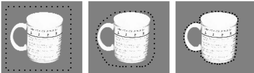
Figure 7: From left to right, images show initial position of the snake. Intermediate position and final position.
