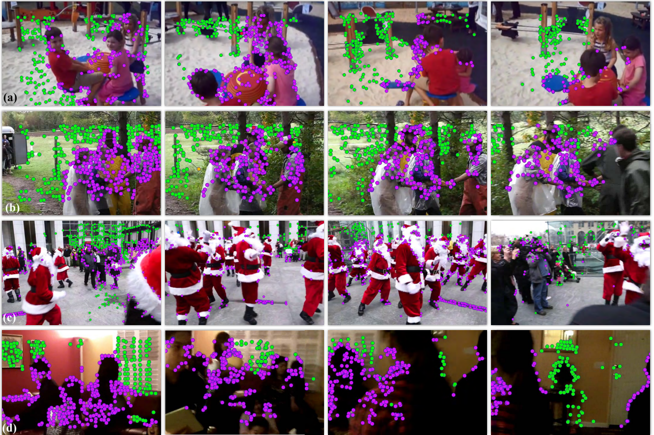
Figure 5: Examples of final selected background feature points, showing as green. Pink points are classified as non-background.
