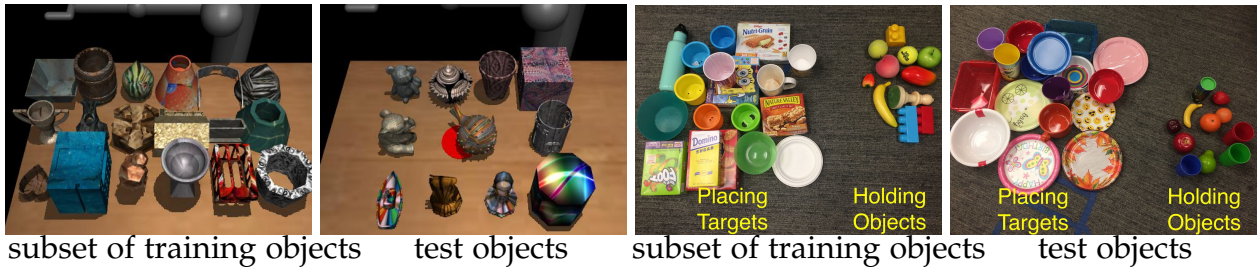
Figure 26: Training and test objects used in our simulated pushing (left) and real-world placing (right) experiments. Note that we only show a subset of the \sim 100 training objects used for the pushing and placing experiments, and a subset of the textures and object scales used for training and testing robot pushing.
