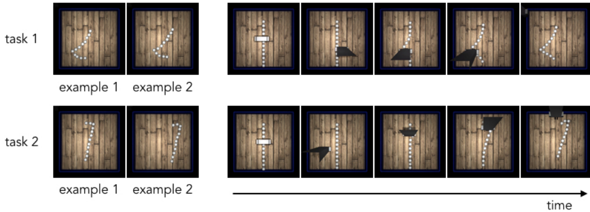
Figure 43: Rope manipulation policy roll-outs. Left: a subset of the 5 positive examples provided for inferring the goal classifier. Right: the robot executing the policy learned via RL with the learned objective.
