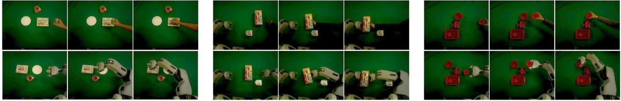
Figure 31: Example placing (left), pushing (middle), and pick-and-place (right) tasks, from the robot’s perspective. The top row shows the human demonstrations used in Section 7.2.7.1, while the bottom shows the robot demonstration.
