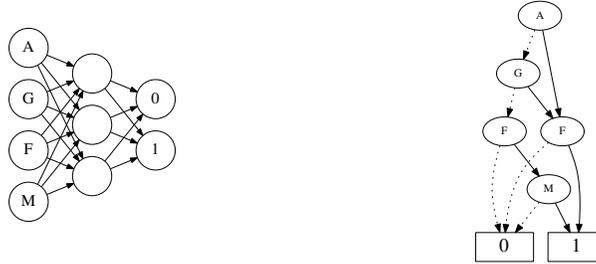
(a) BNN with two outputs  $\{0, 1\}$ . The output with higher activation is the classification.
