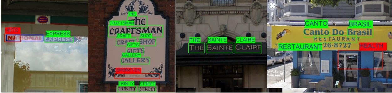
Figure 5. Example output bounding boxes of our end-to-end system on I-FULL and SVT benchmarks. Green: correct detections. Red: false positives. Blue: misses.
