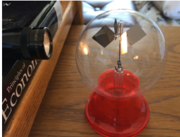
Figure 1, Experiment of a flashlight focused a vane of a Crookes radiometer.
