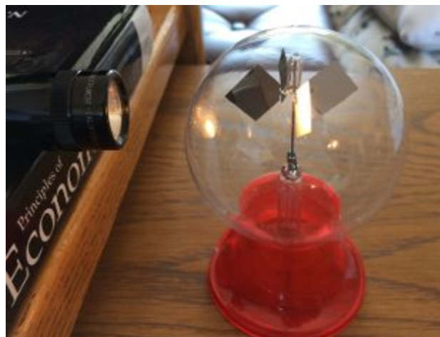
Figure 1, Focused light source experiment for the Crookes radiometer.
