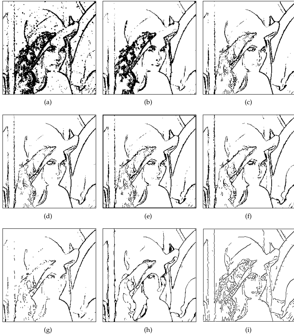
Figure 9: Edge detection result for Lena image in Fig. 8(d): (a) MG detector; (b) amoeba MG detector; (c) BM detector; (d) amoeba BM detector; (e) ATM detector; (f) amoeba ATM detector; (g) RNM detector; (h) amoeba RNM detector; (i) Canny detector
