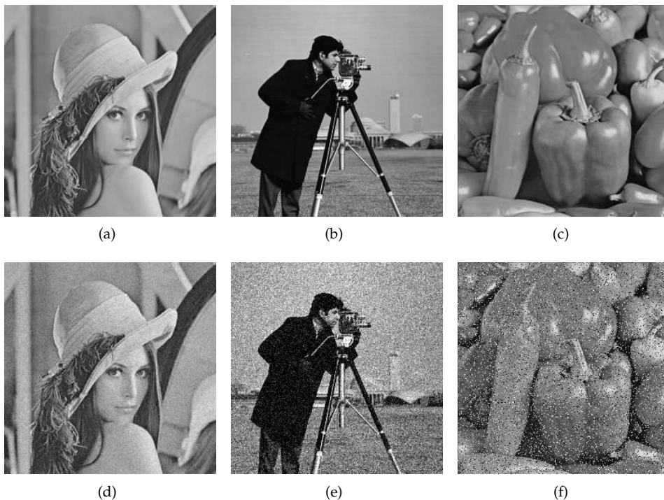
Figure 8: Images used in experiments: (a) Lena; (b) Cameraman; (c) Peppers; (d) Lena image corrupted with Gaussian noise with \sigma = 10 ; (e) Cameraman image corrupted with Gaussian noise with \sigma = 30 ; and (f) Peppers image corrupted with 20% impulse noise
