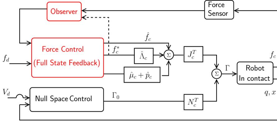
Fig. 2. A block diagram of the contact control framework for a manipulator, where the Active Observer (AOB) design is implemented for force control. The observer in the AOB design includes a state for input disturbance and the estimate of this state will be directly compensated for in addition to the full state feedback.
