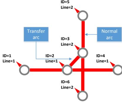
Figure 3. Two types of arcs in the simulation model
