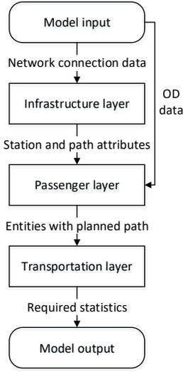
Figure 1. Overall structure of the metro system simulation model
