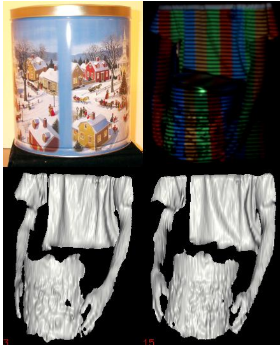
Figure 3.9: Photograph of popcorn tin (upper left), image from sensor camera (upper right), and range maps of person moving a popcorn tin (bottom)
