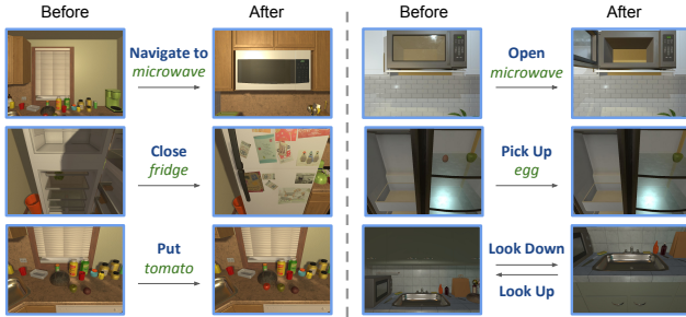
Figure 2. Example images that demonstrate the state changes before and after an object interaction from each of the six action types in our framework. Each action changes the visual state and certain actions may enable further interactions such as opening the fridge before taking an object from it.
