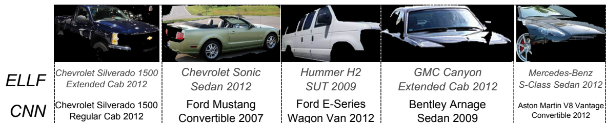
Fig. 6. Example failure cases of ELLF. Incorrect predictions are colored gray and in italics. Part detection for ELLF suffers when GrabCut produces an incorrect segmentation, either by segmenting out too much of the target car or by keeping too much of the background.
