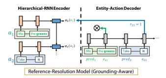
Figure 5: We propose an entity-action pointer network for reference resolution (Sec. 3.4). A hierarchical RNN encodes *action* nodes from language components. Later, we decode grounding-aware *entity* embeddings, where the output "points" to the referring action, if present.
