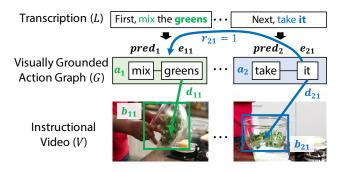
Figure 2: A visually grounded action graph (G) is an action graph with object box nodes  $b_{ik}$  and the corresponding grounding edges  $d_{ij}$  to model the visual grounding of the entities  $e_{ij}$ . This graph serves as the joint representation between the visual grounding within actions  $a_i$  and reference resolution  $r_{ij}$  between them. This reformulates visual grounding and reference resolution as finding the best set of edges (D, R) in the graph given the nodes. See Section 3.1.
