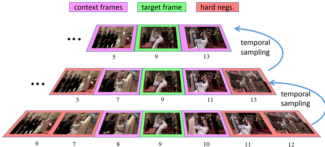
Figure 7.3: Multi-resolution sampling and hard negatives used in our full context model ( T = 1 ). For a target frame (green), we sample context frames (magenta) at varying resolutions, as shown by the rows in this figure. We take hard negatives as examples in the same video that fall outside the context window (red).
