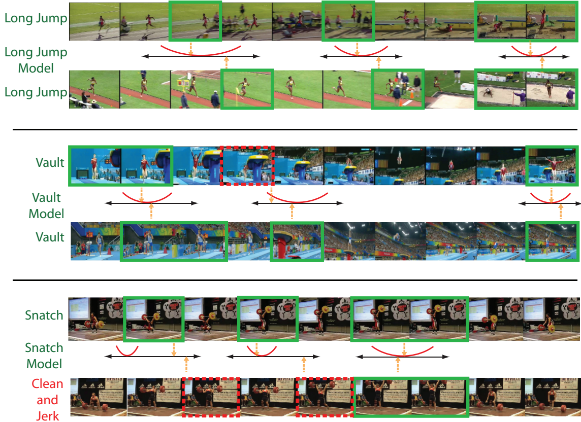
Figure 12.5: Illustration of matching between learned action models for long jump, vault and snatch and some testing sequences. Each group depicts two testing sequences (top and bottom), as well as an illustration of the temporal displacement penalty parameters (middle). Green boxes surround matched temporal segments that are most compatible with the corresponding motion segment classifiers. Red boxes indicate temporal segments that are matched to the motion segment model with a low matching score. The arrows indicate the automatically selected best placement for each motion segment
