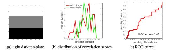
Figure 7.4: Light top dark bottom correlation analysis. (a) Two horizontal layers constituted this template, the top consisting of high-intensity pixels, and the the bottom of low-intensity pixels. (b) A two-dimensional correlation was performed between each image in the dataset and the template. The correlation coefficient for each image was used for classification. (c) shows the classification results in ROC curve. Only a 47.5% performance is achieved by using the template method.
