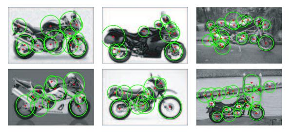
Figure 11.3: The training images for the motorbike category, with the output of the feature detector overlaid.
