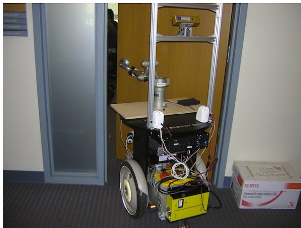
Figure 5.1: STAIR robot platform manipulating a door during one of our experiments.
