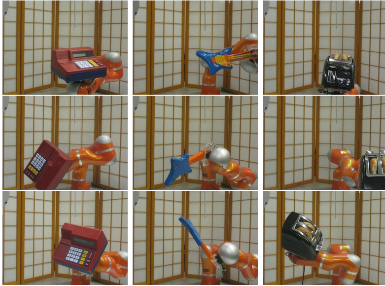
Figure 2.5: The nine poses used during localization experiments (three poses per object). These poses were selected randomly from the uncertainty region. The poses in the top row were also used to run object manipulation scenarios (see videos). All pictures were taken from the same vantage point.
