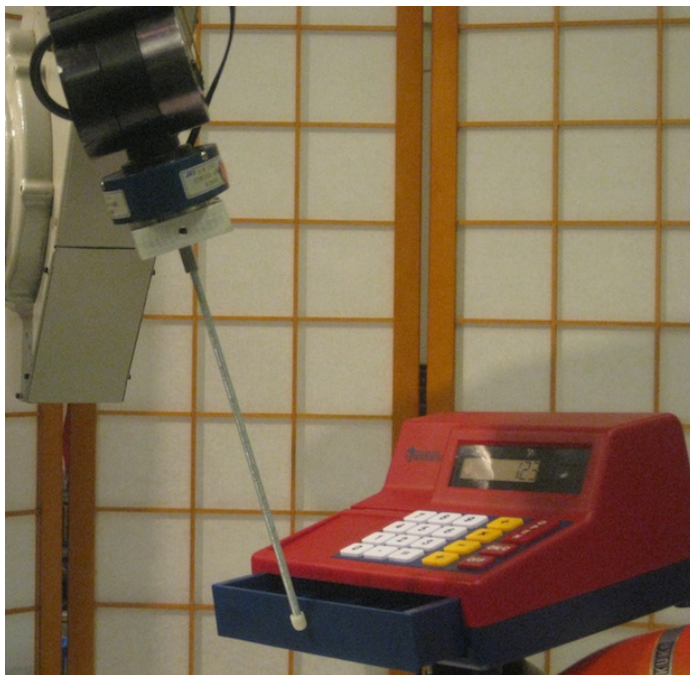
Figure 2.1: In our experiments robots manipulate objects based solely on the sense of touch. Global initial uncertainty is assumed in 6DOF. The photo shows the robot interacting with one of the five objects used in our experiments: the cash register.
