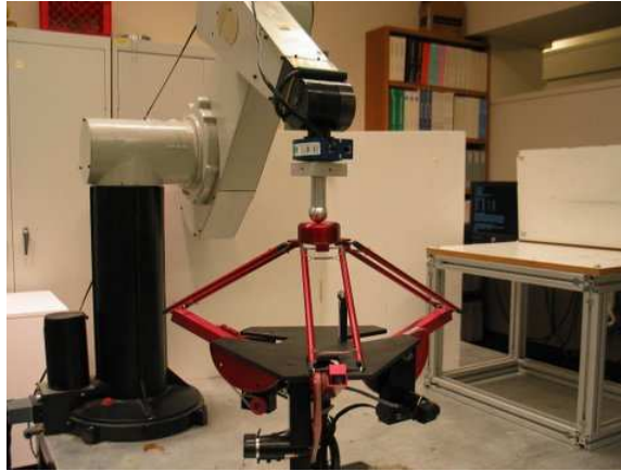
Figure 2.9: PUMA560 in contact with DELTA. A DELTA haptic device is programmed to have a specified stiffness.
