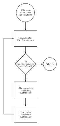
Figure 7. Actuator selection heuristic.
