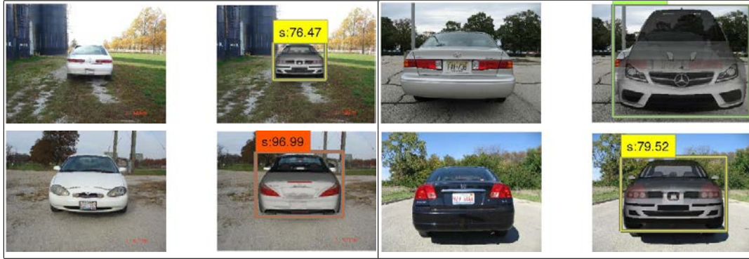
Figure 4: Failed detection or pose estimation on 3D Object Classes [2] cars. Original image (left) and overlaid detection result (right).
