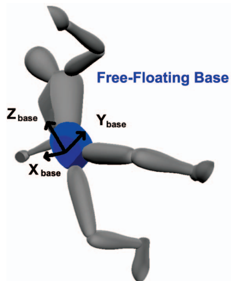
Fig. 1. Free-Floating Humanoid Robot: A free-floating base frame is assigned to the hip link.
