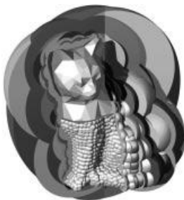
Figure 10. Bounding sphere hierarchy of a cat model.
