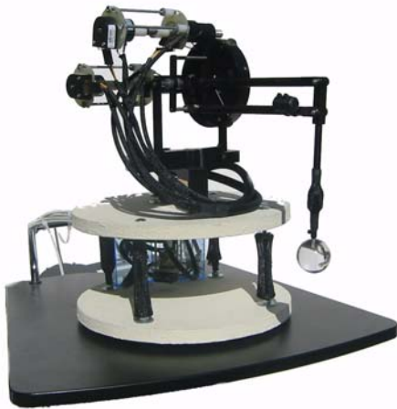
Fig. 9 - Overview of the Stanford Hybrid Haptic Device, which is powered by three hybrid actuator modules that are illustrated in Fig. 10. The device is compensated for gravity by using several counterweights which are positioned along each link.
