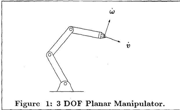
Figure 1: 3 DOF Planar Manipulator.
