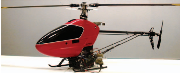
Fig. 4. XCell Tempest: length 135 cm, height 51 cm, weight 5.10 kg, main rotor blade length 720 mm.
