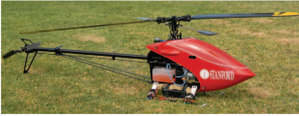
Fig. 5. Synergy N9: length 138 cm, height 40 cm, weight 4.85 kg, main rotor blade length 720 mm.
